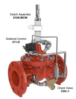
The CLA-VAL SERIES 60 Pump Control Valve is a pilot-operated valve designed for installation on the discharge of pumps to prevent pipeline surges caused by starting and stopping of pumps.
