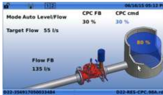
The D22 Home Screen showing the application layout, the relevant feedback and command outputs, plus the mode of operation and target setpoint
