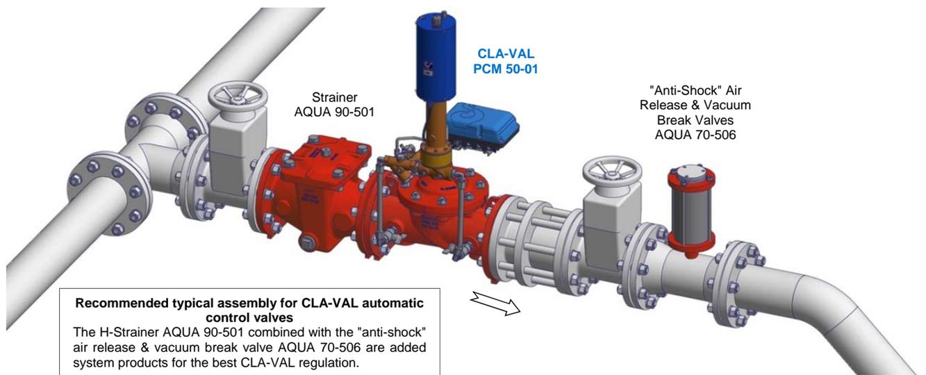
**Recommended typical assembly for CLA-VAL automatic control valves**
