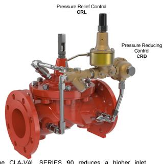
The CLA-VAL SERIES 90 reduces a higher inlet pressure to a constant downstream pressure (Pressure Reducing Control) regardless of changing flow rate and/or varying inlet pressure.
