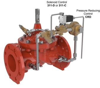
The CLA-VAL SERIES 90 reduces a higher inlet pressure to a constant downstream pressure (Pressure Reducing Control) regardless of changing flow rate and/or varying inlet pressure.
