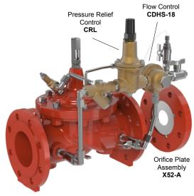
The CLA-VAL SERIES 40 is used to accurately limit excessive flow to a preselected maximum rate (Flow Control) regardless of changes in pressure and/or varying inlet flow.
