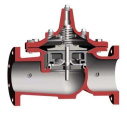
The CLA-VAL Model 100S/2100S Seawater Service Hytrol Valve is a hydraulically operated, diaphragm actuated, globe or angle pattern valve. It consists of three major components: body, diaphragm assembly and cover. The diaphragm assembly is the only moving part.
