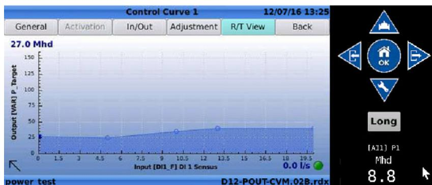
This screen illustrates that as the flow increases, the motorized control pilot will increase the output pressure according to the graph.
