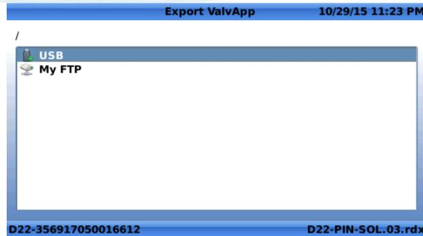
When exporting the application to the server, the \*.rdx file will be pushed to the FTP server configured in the Electronic Controller in the "SYNClUP" folder.
