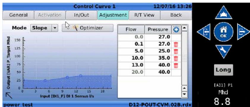
The control curve can be completely customised by inserting the required values in the table of the "Adjustment" tab.
