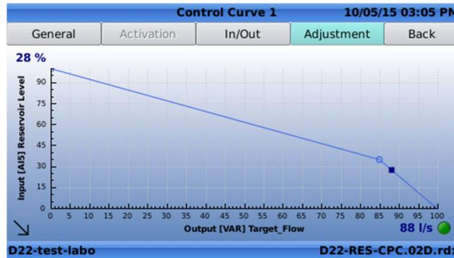
This screen describes that as the reservoir level decreases, the targeted flow (to fill the reservoir) increases, and the motorized control will act accordingly.
