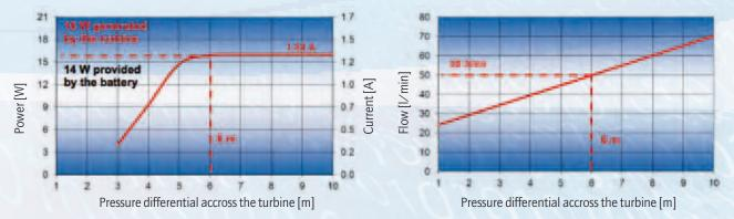
Note : The power showed in the graphs is obtained by optimising the power generated by the turbine for each pressure differential.
