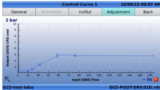
This screen describes that as the flow increases, the motorized control will increase the output pressure up according to the graph.
