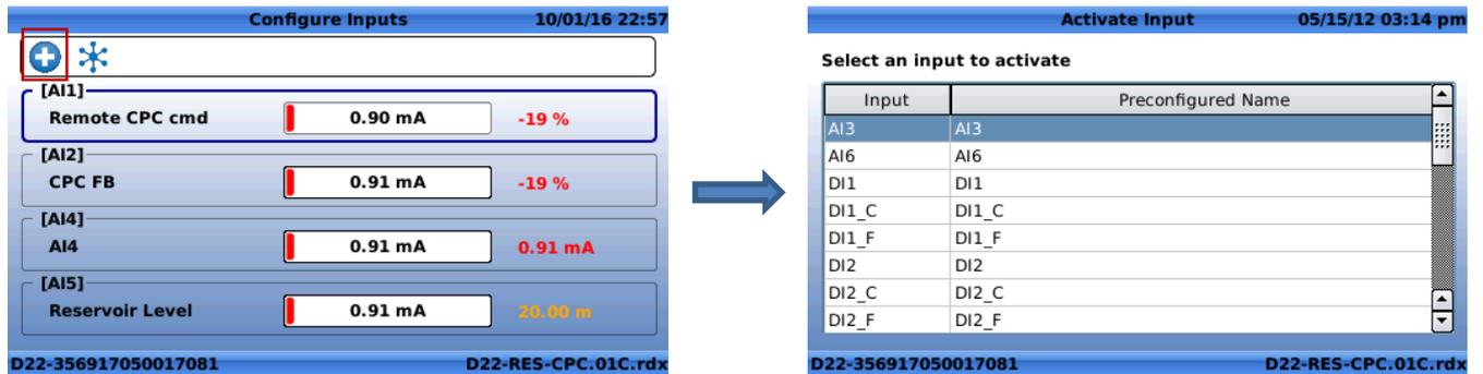
By clicking the "+" button, the input to be activated can be chosen from the list. The input added will then show up in the list of input of the configuration screen.
