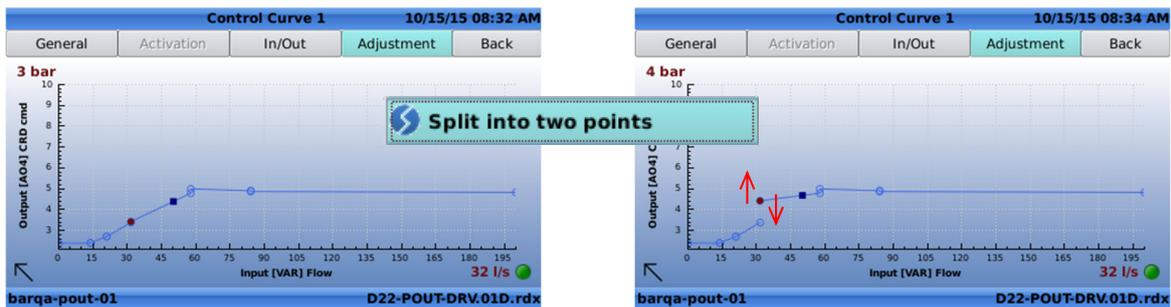
After the point is split, it can be moved up or down using the and buttons.
