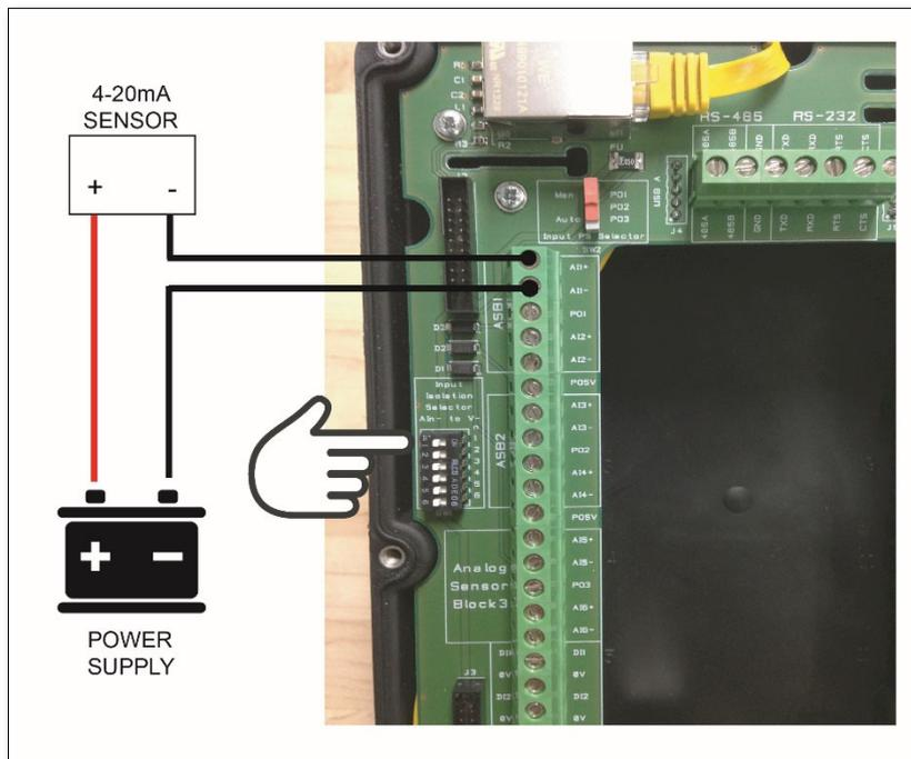
For isolated 2-wire signals, the power supply, sensor and Electronic Valve Controller make a continuous loop, allowing the current to be measured by the Electronic Valve Controller.
