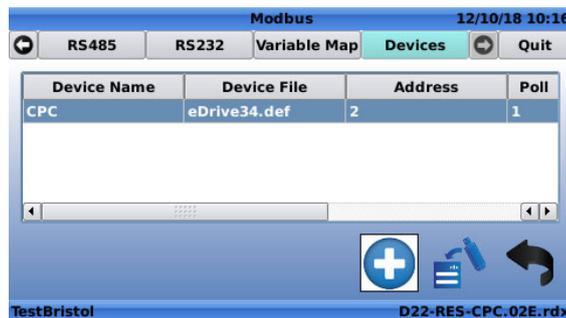
Once the actuator is interfaced to the Electronic Valve Controller advanced controller, the following e-Drive-34 signals are available:
