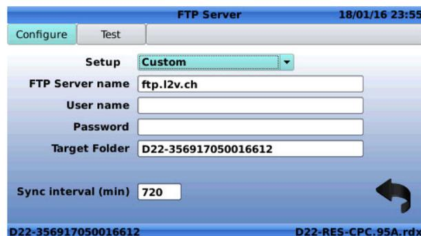
The screenshot shows the 'FTP Server' configuration interface with the 'Setup' dropdown menu set to 'Custom'. The 'FTP Server name' field contains 'ftp.l2v.ch'. There are fields for 'User name' and 'Password'. The 'Target Folder' field contains 'D22-356917050016612'. The 'Sync interval (min)' is set to '720'. At the bottom, the device ID 'D22-356917050016612' and the file path 'D22-RES-CPC.95A.rdx' are displayed.
