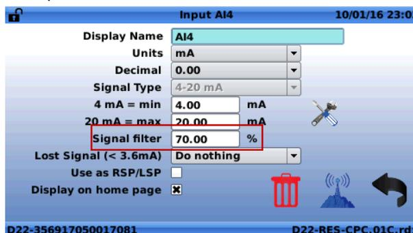
The value can be set from 1% (light) to 99% (strong) or disabled. The default value is set at 70%, which is usually a good filtering for most of the application.
