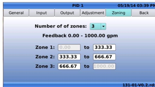
The screenshot shows the 'Zoning' tab for 'PID 1' on 05/19/14 at 03:39 PM. The 'Number of zones' is set to 3. The feedback range is 0.00 - 1000.00 gpm. The zones are defined as follows: Zone 1 (0.00 to 333.33), Zone 2 (333.33 to 666.67), and Zone 3 (666.67 to 1000.00). The file path 131-01-V0.2.rdx is visible at the bottom.
