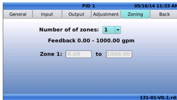
The screenshot shows the 'Zoning' tab for 'PID 1' on 05/16/14 at 11:33 AM. The 'Number of zones' is set to 1. The feedback range is 0.00 - 1000.00 gpm. Zone 1 is defined from 0.00 to 1000.00. The file path 131-01-V0.1.rdx is visible at the bottom.
