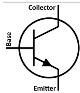
An NPN transistor can be used as a digital input because the state is either open (V+) or closed (V-). Depending on how the input is configured, action can be taken when this NPN transistor switches state.
