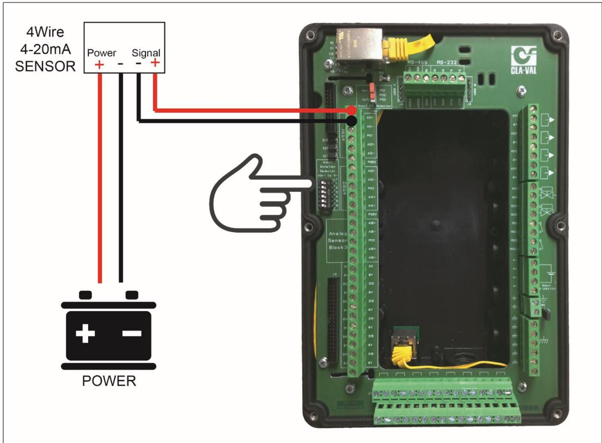
For 4-wire signals, the Sensor is externally powered usually using 2 wires. The two signal wires coming from the sensor are then measured by the Electronic Valve Controller in the Analog Input section of the terminal board.
