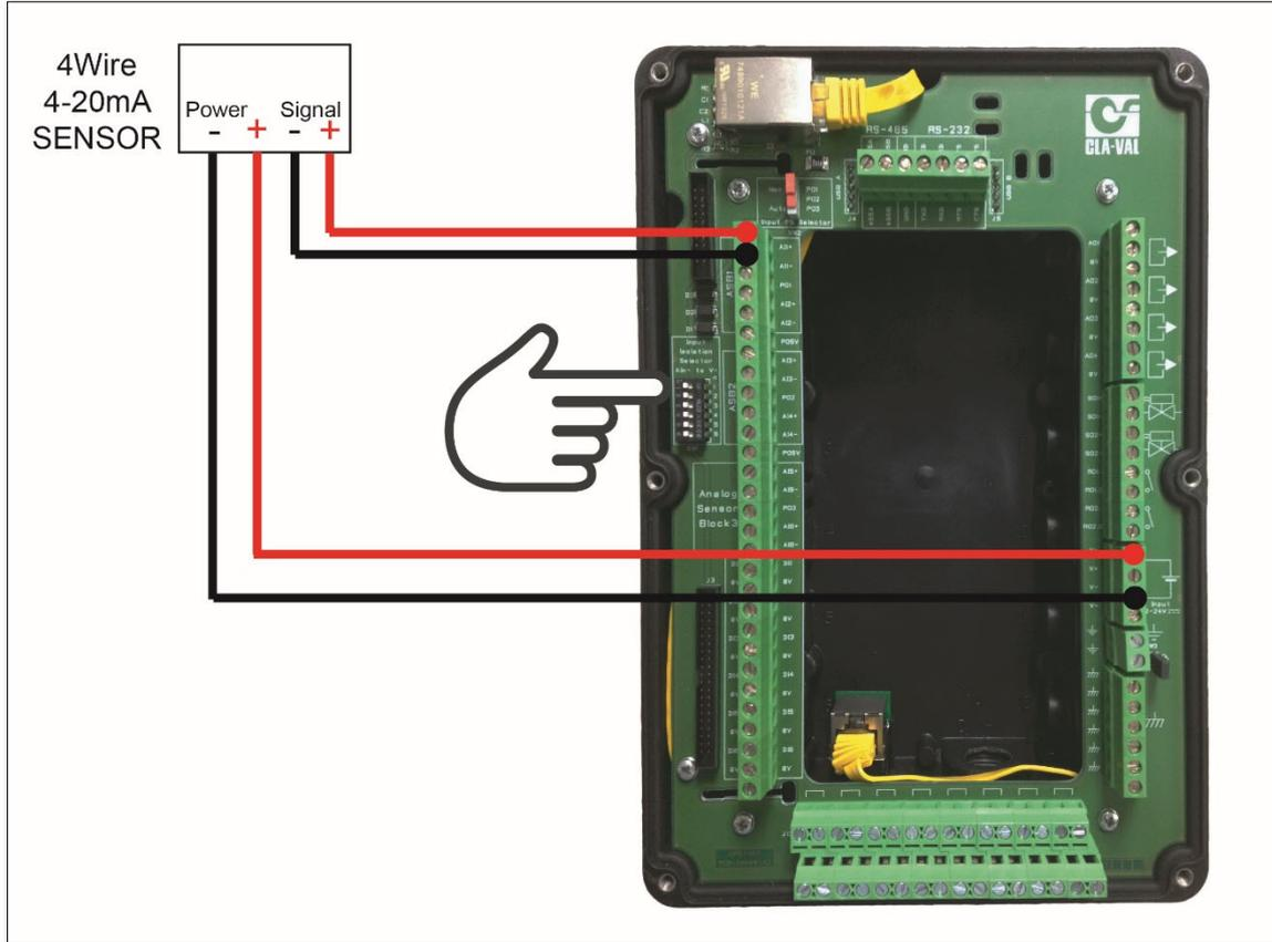
For 4-wire internally powered signals, the sensor is powered directly from the main Electronic Valve Controller power supply terminals. The two signal wires coming from the sensor are then measured by the Electronic Valve Controller in the Analog Input section of the terminal board.
