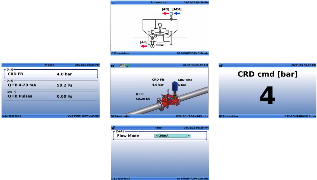
A) "Inputs": The Inputs menu displays all of the activated inputs in current use by the selected *ValveApps™*.
