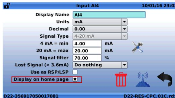
An added input can be deleted by clicking on the trash icon of the same screen.
