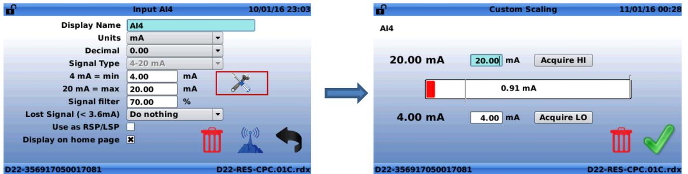
Push "Acquire Lo" to set the minimum value and "Acquire HI" to set the maximum value, and validate with the check mark. Note that the sensor can also have a reversed range, i.e. minimum physical value for 20 mA and maximum physical value for 4 mA.
