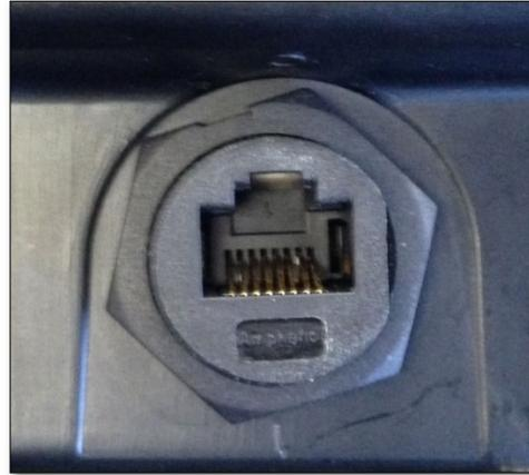
The Ethernet port 100 Base-T (right) accepts standard RJ-45 Ethernet cables (left).
