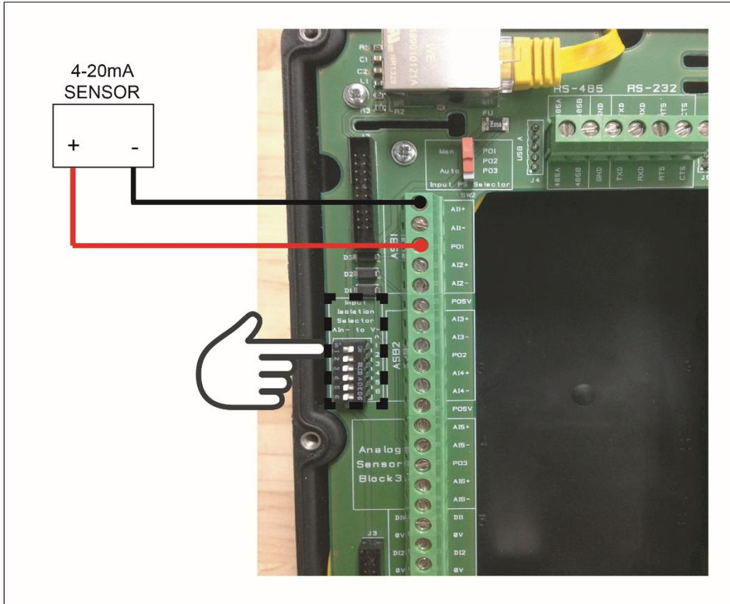
For non-isolated signals, the Electronic Valve Controller provides the power for the sensor and makes a continuous loop, allowing the current to energize the sensor and then be measured by the Electronic Valve Controller.
