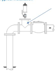
Recommended air accumulator min 0.5 x diameter of riser main.
