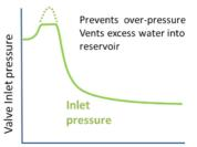
The Cla-Val Series 138L-36 provides remote management of reservoir level with hydraulic pressure sustaining control to protect upstream pipework from low pressure.
