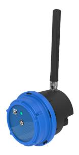
**CLA-VAL CV-Log-35** is an ultra-low power smart data logger with 6 acquisition channels (4 analog and 2 digital inputs). Acquired data is stored in a large internal memory and can be transmitted through the 4G LTE-M and NB-loT communication networks, optimized for data communication. The product is also compatible with legacy 2G (GPRS) networks.
