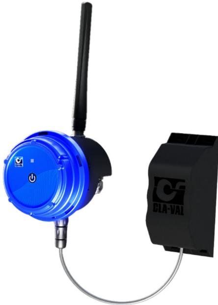
**CLA-VAL D35** is an ultra-low-power autonomous electronic valve controller switching one or two latching solenoids based on customizable conditions to control valves in locations where no electrical energy is available or independent supply from grid power is required.
